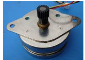
Figure 8.67 AIRPAX LB82773-M1 bipolar stepper motor
