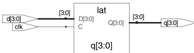
Figure 4.19 latch synthesized circuit
