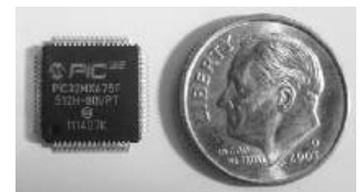
Figure 8.32 PIC32 in 64-pin TQFP package
