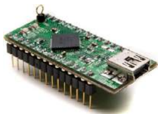
Figure 8.76 FTDI UM232H module (© 2012 by FTDI; reprinted with permission.)
